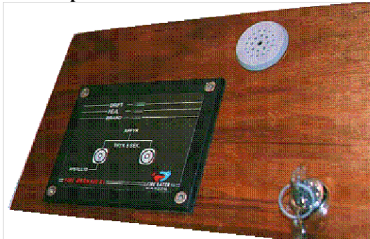
Sounder at top corner and ignition switch in lower right corner.
