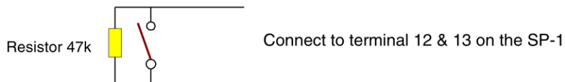
General connection of Normally Open Alarm (NO) Contacts to Loop 1 of the SP-1
