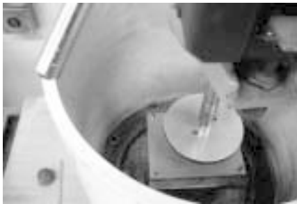
Figure 7.4—Disc and wear plates mounted onto test stand.
