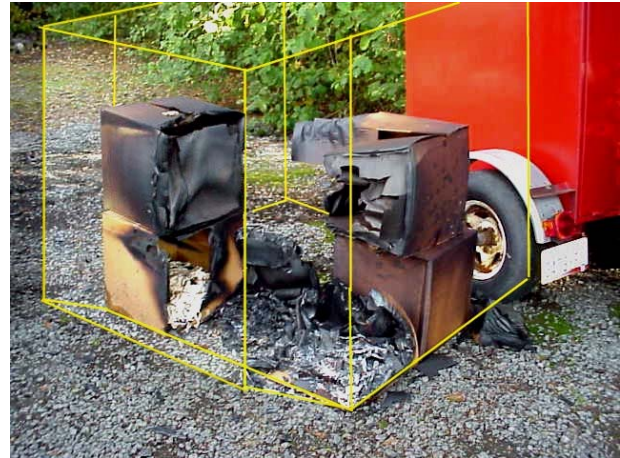
Figure 11 a. Post Fire damage to the containerized fire load b. Damaged boxed reconstructed
